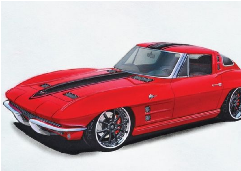
This is an artist's rendition of the '63 split-window Corvette that Tony Arme and his crew are working on. It includes such touches as mesh screens on the hood and front-quarter panels that evoke the newest Vettes. The original plan was to put an LS3 V-8 under the hood; that changed when Chevy introduced the 6.2-liter LT1. (Photo: Paul Kuras)
